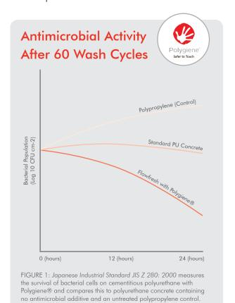
The Polygiene® additive is homogenously distributed throughout the Flowfresh system, which means that, unlike synthetic antimicrobial additives or surface treatments, it remains active for the lifetime of the floor even if worn or damaged. Therefore, should a Flowfresh floor's surface become damaged, any germs within the gap will still be exposed to the active antibacterial agent.
